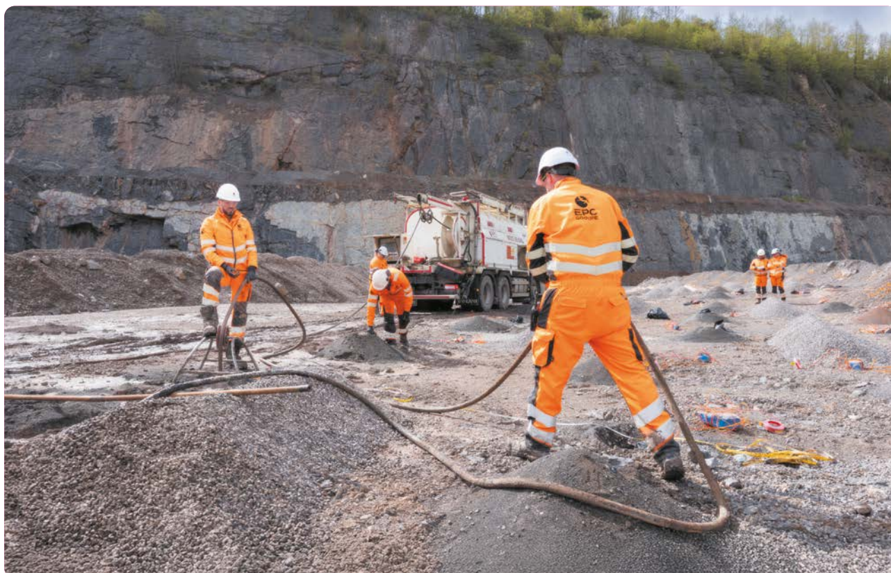
Preparation of a blast
